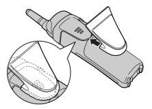
To remove the shoulder rest attachment Slide the base of the attachment.
