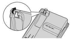
2 Press the tabs in the direction of the arrows (①), then remove the wall mounting adaptor (②).
